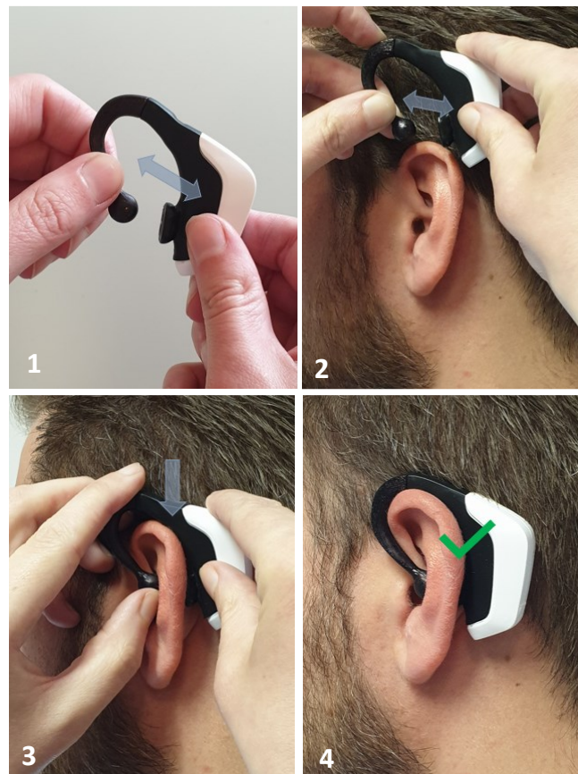
Figure 26 - Attaching the EarSensor to the patient
