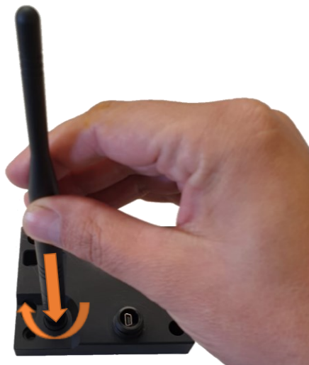
Figure 7 – Connecting antenna on coordinator
