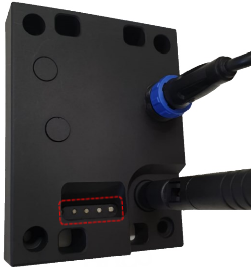
Figure 51 - Location of the status LED's of the Coordinator
