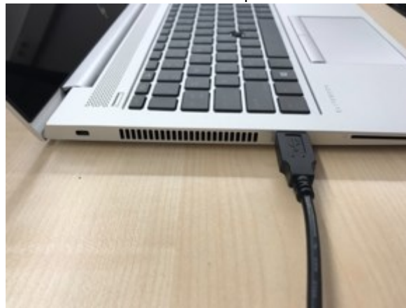
Figure 9 – Connect the Coordinator to the laptop.
