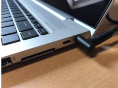
Figure 5 – Connect the power supply to the laptop.
