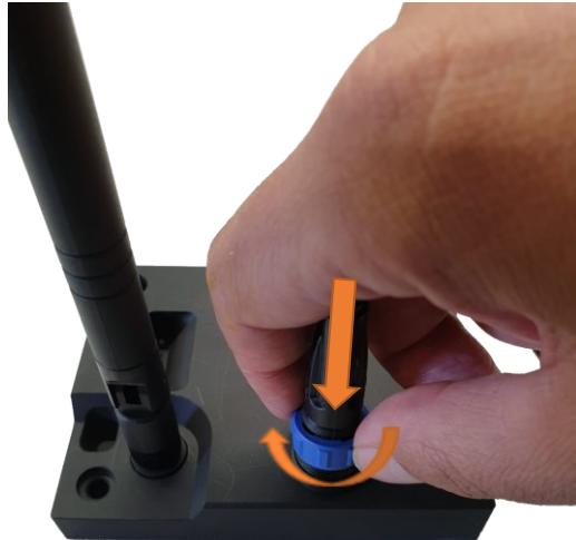
Figure 8 - Connect USB cable to Coordinator
