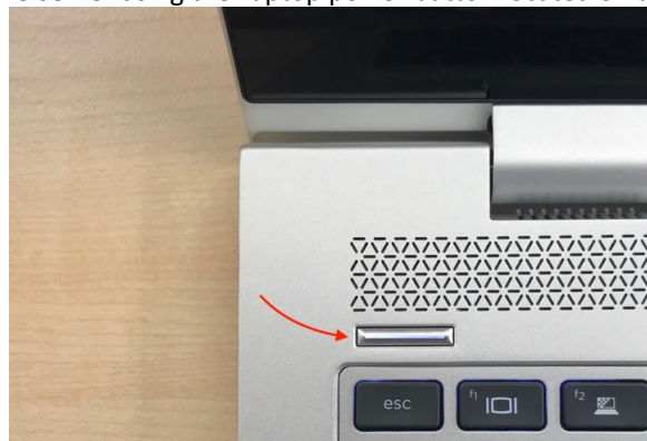
Figure 10 – Turn on the Server using the Laptop power button
