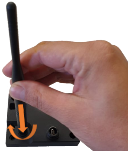
Figure 7 – Connecting antenna on coordinator.
