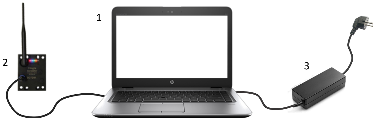
Figure 3 – Server module including laptop, Coordinator, and power supply.
